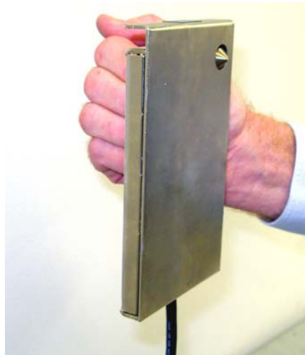
VDA backer plate Contacts specimen on entire surface
