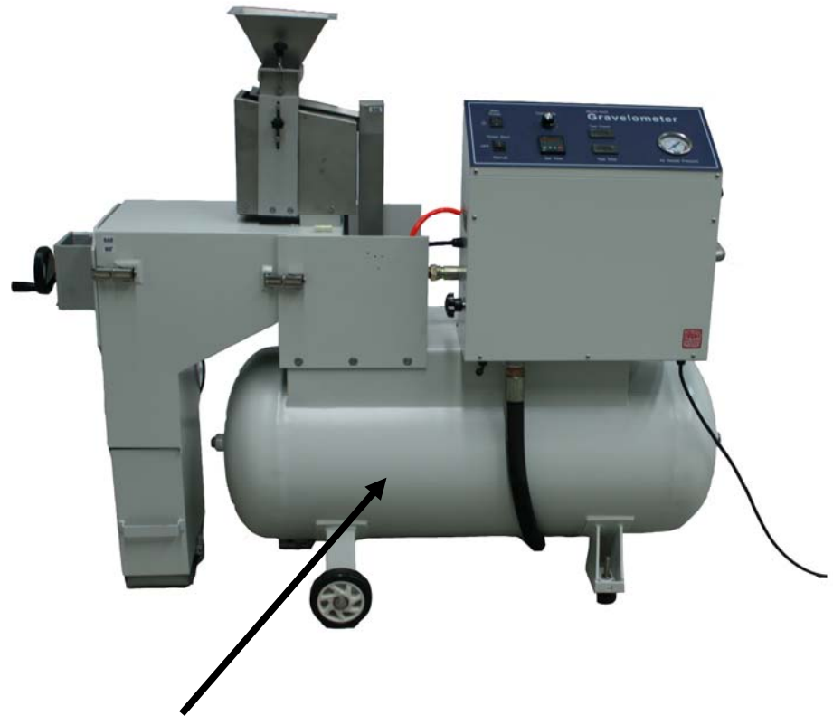
Gravelometer and Air Receiver Tank
