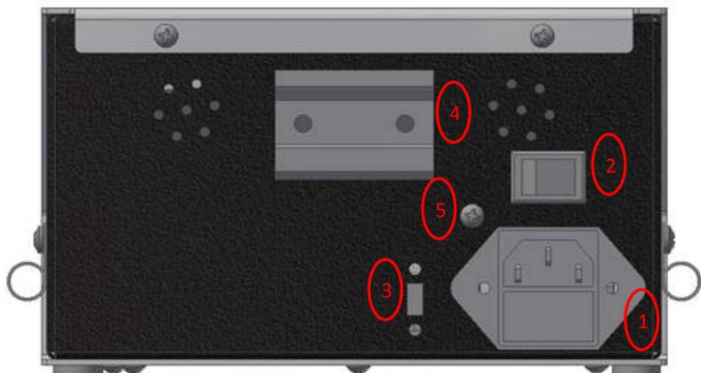
4. **Grid Bracket Holder** - This can be used to mount the device. It allows the device to swivel up or down on a horizontal bar to allow for optimal viewing angle of the display.
