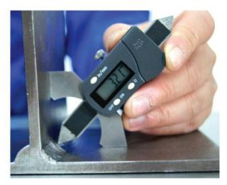
**Weld Measuring Gauges** permit you to accurately check welds of varying sizes quickly and easily. You can measure Weld Throat Thickness, Butt Fillet Type Welds, Weld Length, Misalignments (High-Low), and much more depending upon the Gauge selected.
