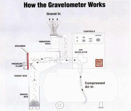
A measured amount of gravel is vibrated out of a hopper and down a feed chute, where a vacuum exists due to the high velocity airflow below. The media is sucked down into the gun assembly and is fired at the test specimen by means of this air blast. After the media hits the target, it falls into the gravel box below.
