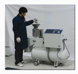
run hundreds of tests per day. It allows quick specimen loading/unloading and features an external gravel box for greater ease of use. The Gravelometer also incorporates enhanced control of test parameters and allows calibration for ISO 9000 compliance.
